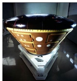
Telemetry antenna with window on ARD (Atmospheric Reentry Demonstrator)
